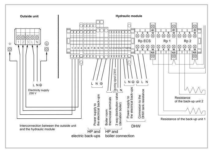
Figure 37 - Connection to terminal block and power relays
