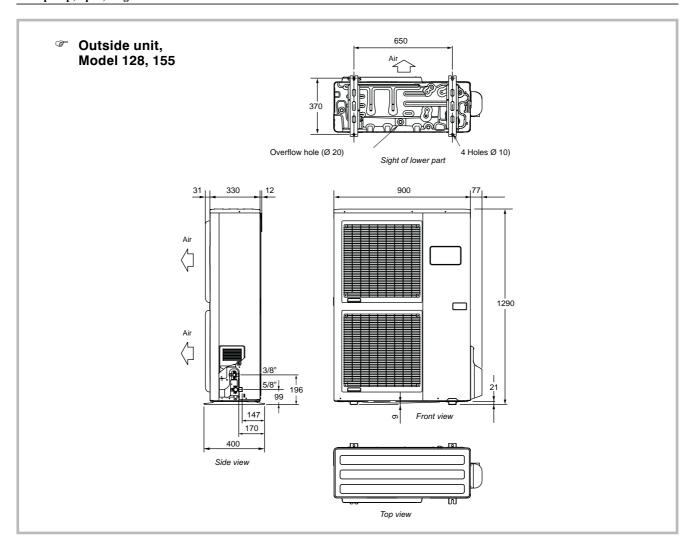
Figure 2 - Dimensions in mm
