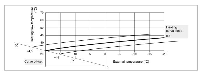
Figure 42 - Off-set of the heating curve (line 721)
