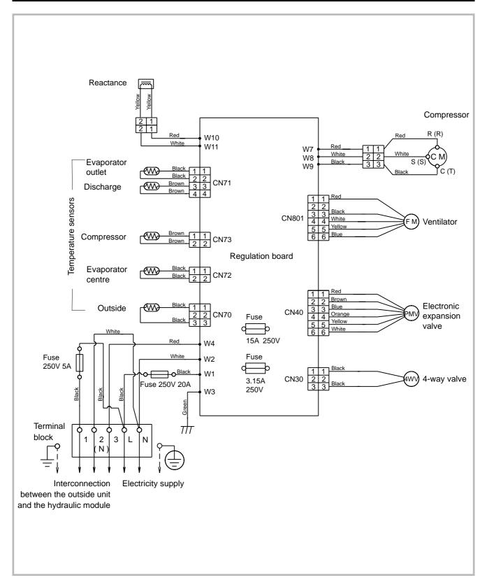
Figure 45 - Electrical wiring of outside unit Model 050, 065, 080
