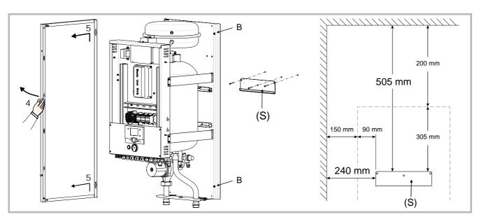
Figure 17 - Removing the sides and fixing the support (S)
