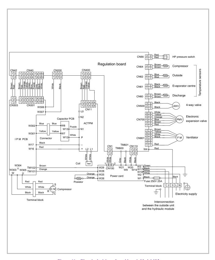
Figure 46 - Electrical wiring of outside unit Model 095
