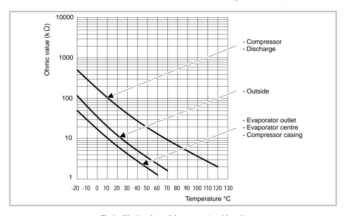
Fig. 6 - Ohmic values of the sensors (outside unit)
