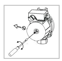
Figure 25 - Release of the circulation pump
