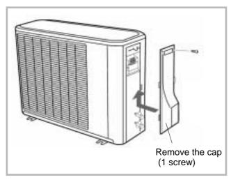
Figure 32 - Access to outside unit's terminal block (model 050, 065, 080)
