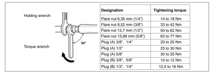
Figure 21 - Tightening torque
