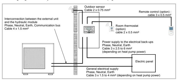
Figure 31 - Overall layout of the electrical connections for a simple installation (1 heating circuit)
