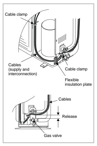
Figure 35 - Finalisation of connection to outside unit
