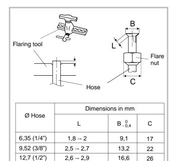
Figure 18 - Flaring for flare connections
