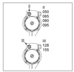
Figure 26 - Recommended circulation speed (for radiator)
