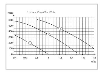
Fig. 4 - Hydraulic pressures and flow rates available
