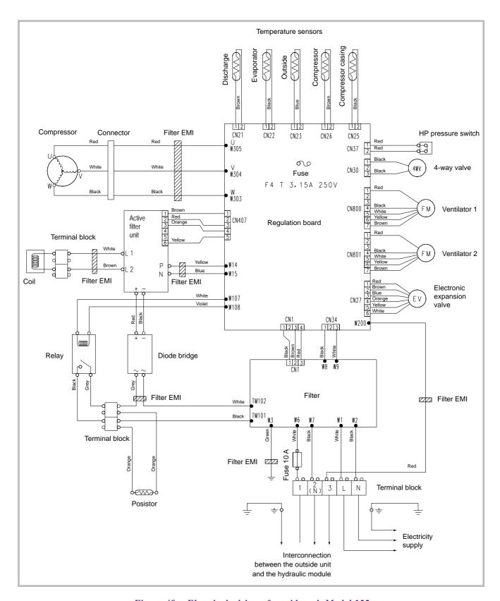
Figure 48 - Electrical wiring of outside unit Model 155
