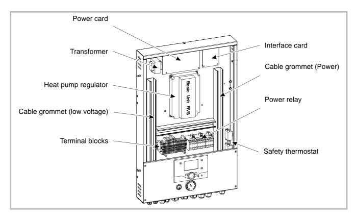
Figure 36 - Access to hydraulic model electric box and description
