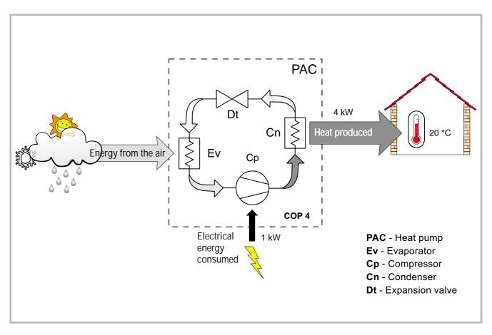
Figure 9 - Heat pump operating principle
