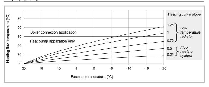
Figure 41 - Heating curve slope (line 720)
