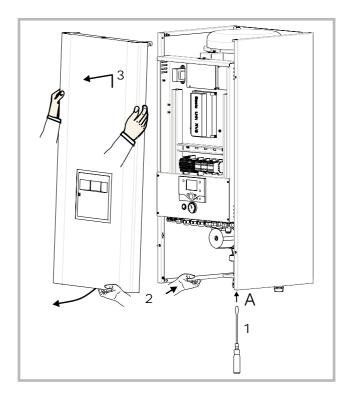
Figure 16 - Removing the front facing
