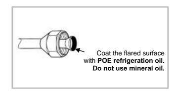
Figure 20 - Prevention of gas leaks
