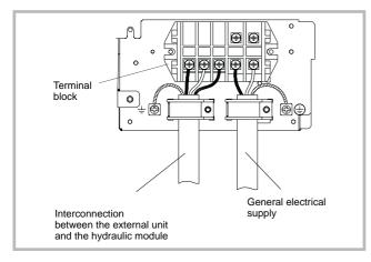
Figure 33 - Connections to outside unit's terminal block
