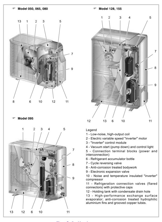
Figure 7 - Outside unit components
