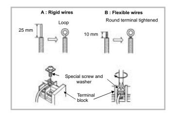
Figure 28 - Outside unit terminal block
