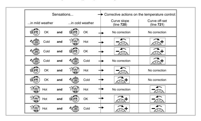
Figure 43 - Corrective actions in the case of discomfort
