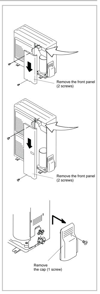
Figure 34 - Access to outside unit's terminal block (model 095, 128, 155)
