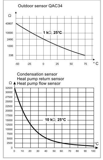
Fig. 5 - Ohmic values of the sensors (Hydraulic module)
