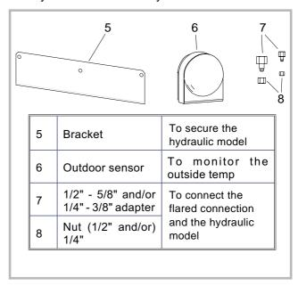
Figure 11 - Accessories provided with the hydraulic module
