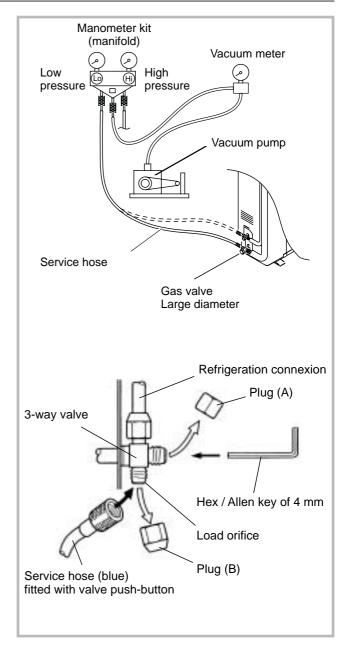
Figure 22 - Extraction under vacuum and gassing
