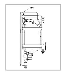
Figure 27 - (P) Hydraulic module bleeder valve
