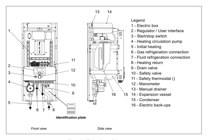
Figure 8 - Hydraulic module components
