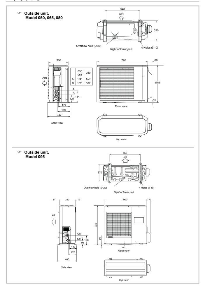
Figure 1 - Dimensions in mm
