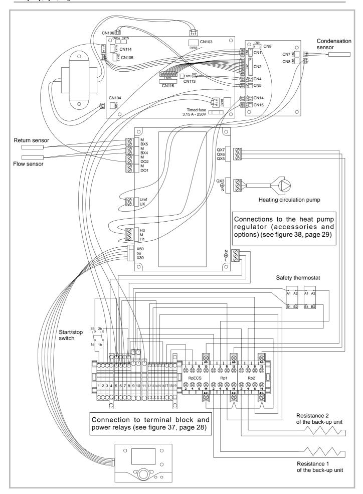
Figure 49 - Electrical wiring, Hydraulic module (Except installer's connections)
