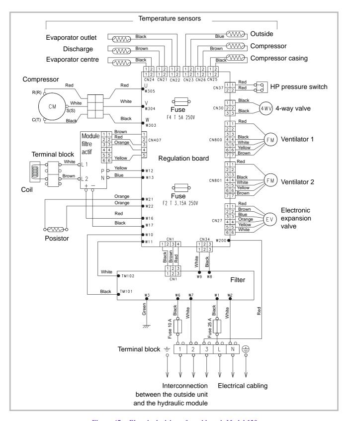
Figure 47 - Electrical wiring of outside unit Model 128
